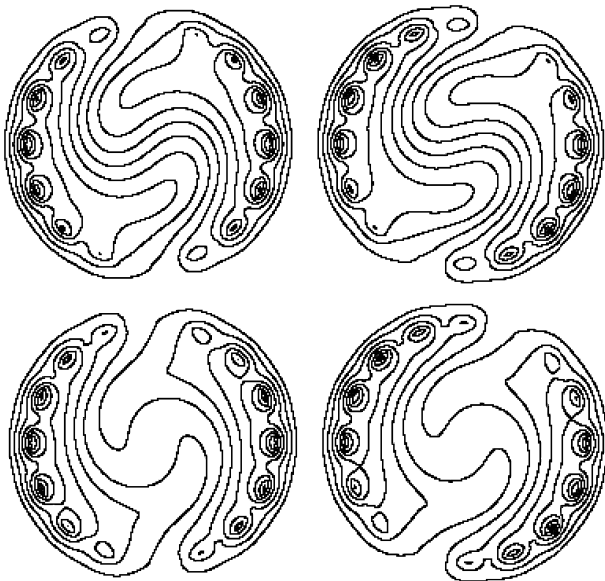
Fig. 6. Similar to Fig. 5, but for dielectric cylinder inside a shielded cylindrical resonator, and at two conditions of damping. Time exposures of CW rotating flux for quadrature excitation at 157 MHz of a lossy dielectric cylinder, of radius 9.25 cm, viewed in a diametral plane, for two conditions of damping: (i) above, left and right, underdamped, Q = 1.0 ( \epsilon = 80 , \sigma = 0.7 ); and (ii) below, left and right, overdamped, Q = 0.35 ( \epsilon = 80 , \sigma = 2 ). The cylindrical resonator is assumed to be bird cage type with 16 elements on a bolt circle of radius 14.6 cm, and a cylindrical shield of radius 17.7 cm. (This matches the dimensions of our experimental resonator.) The current distribution is assumed to be sinusoidal. As in earlier figures of this type, the vector potential points perpendicular to viewing plane so that the iso-contours of vector potential are true flux lines, again, as explained in the legend to Fig. 4.
